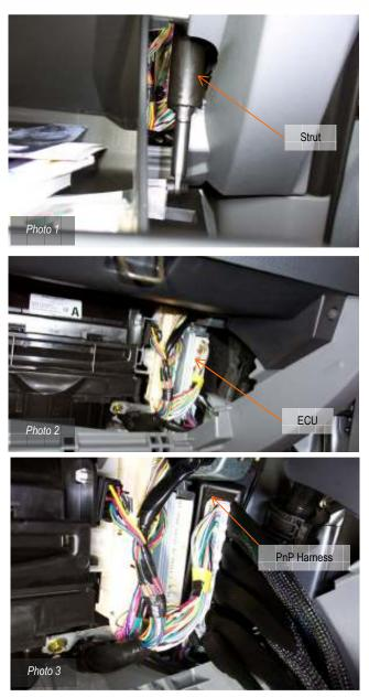
v. (Photo 4) Disconnect OEM plugs 1, 3, 4, and 5 (counting from top-to-bottom) and insert them into the PnP Harness Connectors.
